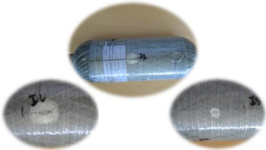
Figure 6.11: Impact defects I1 (top), I2 (bottom left) and I3 (bottom right) on the three layer 2.5 L reservoir.
