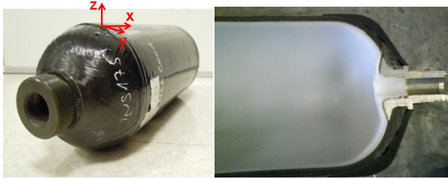
Figure 1.1: Example of a multi-layer composite vessel intended for housing Hydrogen gas at high pressures: overview (left) and sectional view (right).
